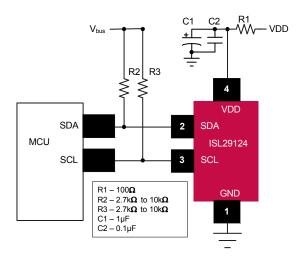
FIGURE 1. TYPICAL APPLICATION DIAGRAM
